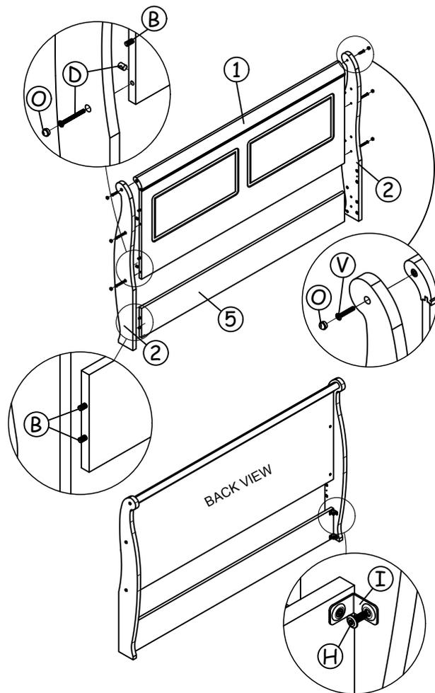
Fix the headboard frame panel (1) and headboard back panel (5) to the headboard wood post (L/R) with hardware parts as shown.
