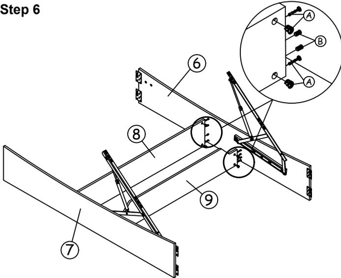
Join together the left side rail (6) and right side rail (7) with the centre storage panels ① (8) and centre storage panels ②(9) by using hardware parts **A** and **B**.
