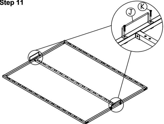
Attach hardware parts **J** using hardware part **K**.
