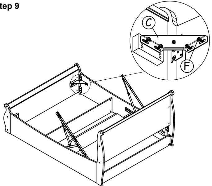
Fix metal corner block **C** to the edge of footboard and side rails with bolt **F** as shown.
