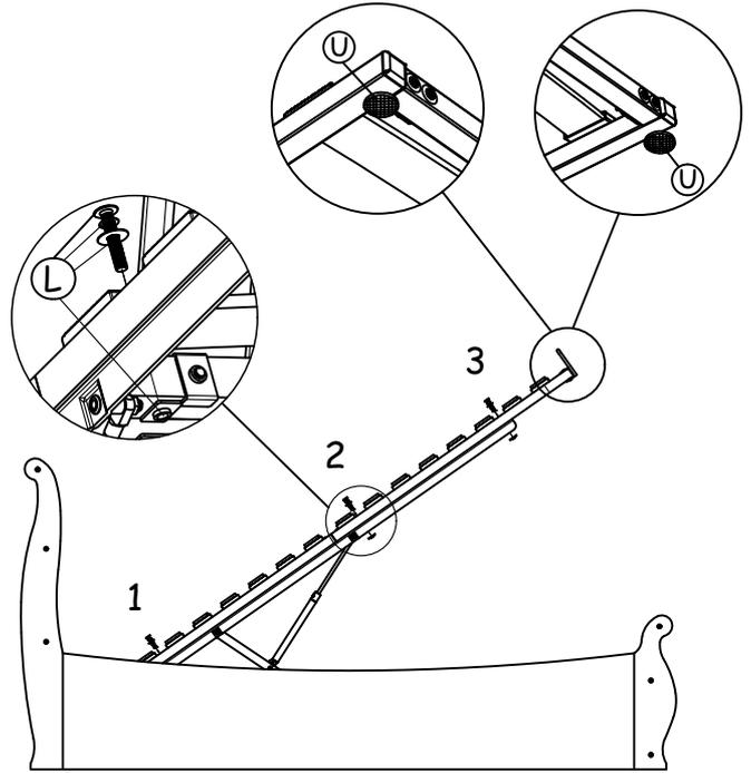
Assemble the bed base on the right & left hydraulic frame and fix bolts **L** starting from '1' to '3' as shown and then stick it the self adhesive **U** as shown.
