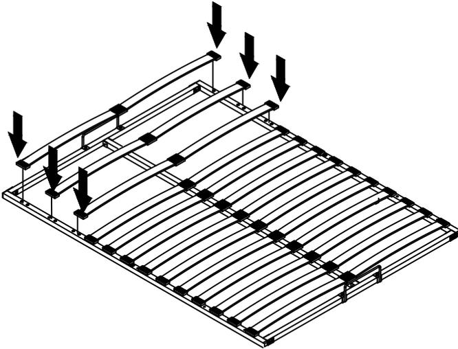
Insert the slats (13) to hardware parts **M** and **N** then press into the base making sure they are secure.
