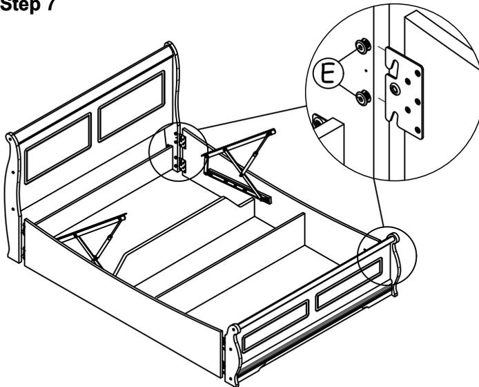
Attach the headboard frame (1) and footboard (4) using hardware part **E** than tighten up.
