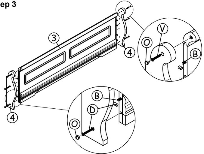
Fix the footboard frame panel (3) to the footboard wood post (L/R) (4) with hardware parts as shown.
