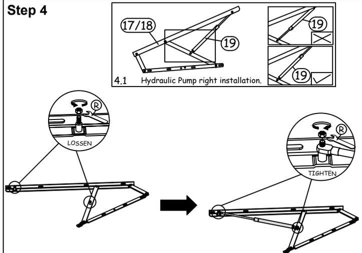
Firstly, Loosen the **Hex Nut** from the Left & Right Hydraulic Base Support ,then fix the hydraulic pump to each hydraulic base using the same **Hex Nut** & **V**. (shown in diagram 4.1. )
