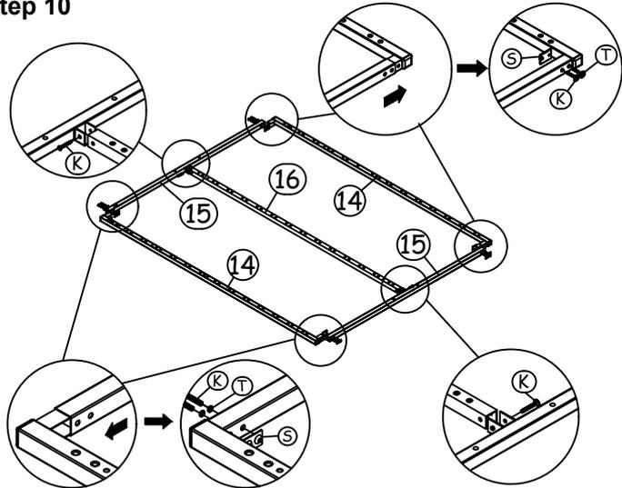
Join together all the bed base parts (14),(15), and (16) by using hardware parts **K,S,T**.
