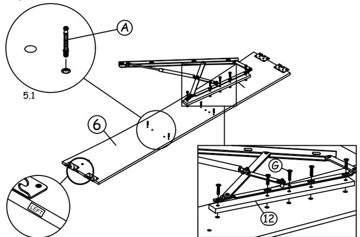
Fix the left & right hydraulic spacer together with hydraulic base supporter to the both side rails using bolts **G** and than screw the minifix part **A** to the both side rails as shown in diagram 5.1.
